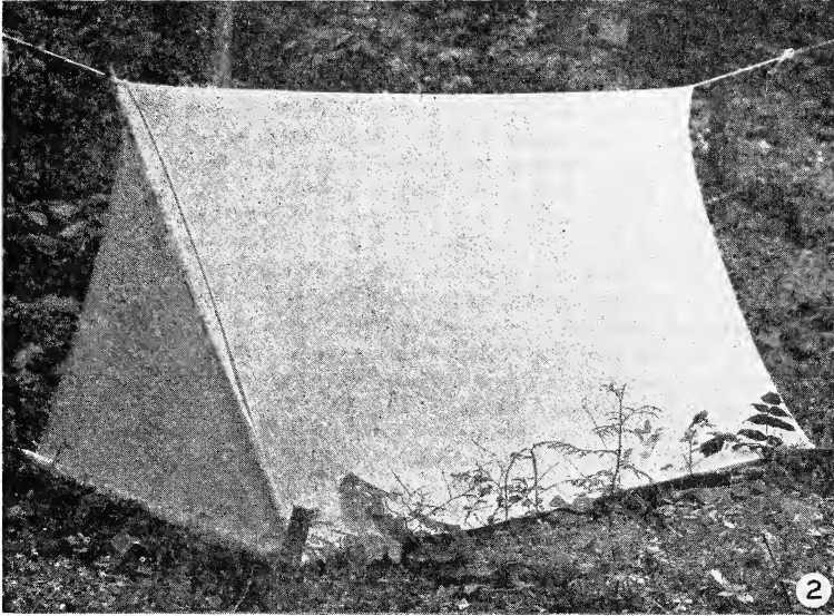
Fig. 1. Nylon-mesh tent-cage showing continuous apex ties and front opening closed by gathering of 3-foot sleeve tied with cord.
